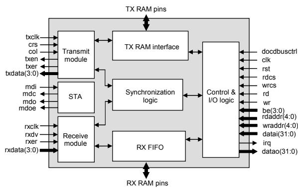
**Transmit module** – Performs transmit management functions, sends frames to Ethernet medium.
