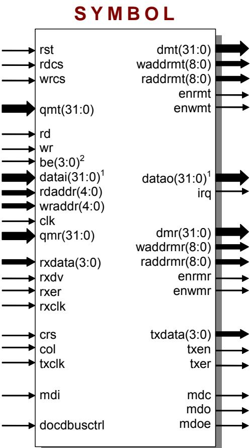
1 – data bus can be configured as 8-, 16- or 32- bit depends on processor's bus size
